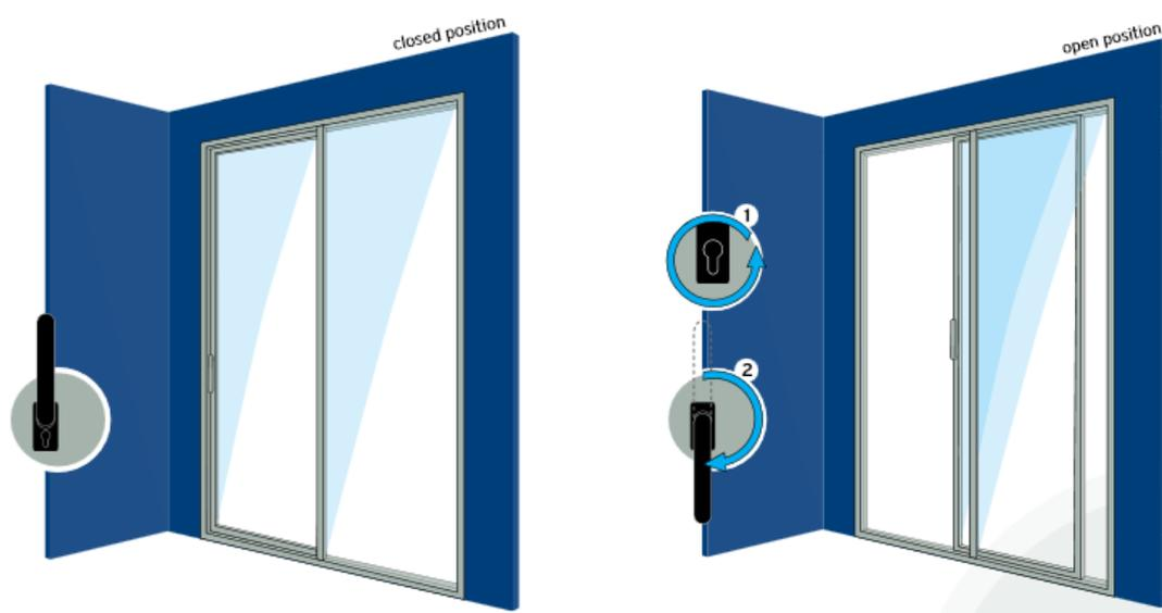
**DO NOT operate** the door with the handle at 90° – the wheels won't be fully retracted and the door will drag on the threshold meaning the gaskets may become damaged and ultimately compromise the weathering performance of the door.
